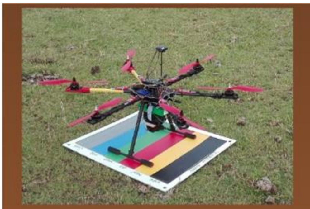
Figure 1. The drone used to capture multispectral data.
